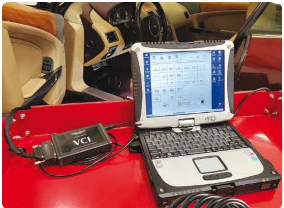
Aston Martin AMDS laptop connected to a DB9
